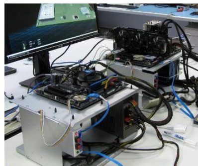
Testing client setup for issue replication and running benchmarks
