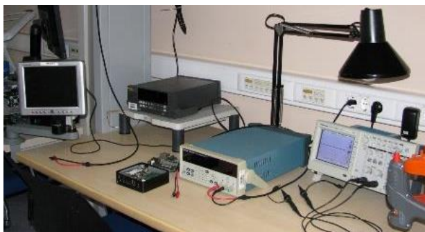
Test-station with oscilloscope for observing the changes of an electrical signals while troubleshooting malfunctioning electronic equipment
